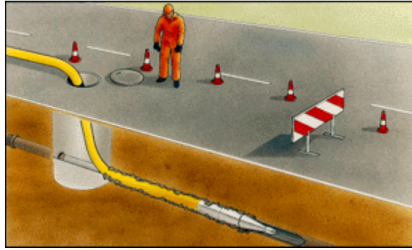
Fig. 5: Pipe Bursting System.
